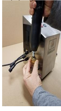
Hose to Control Box/Pump
